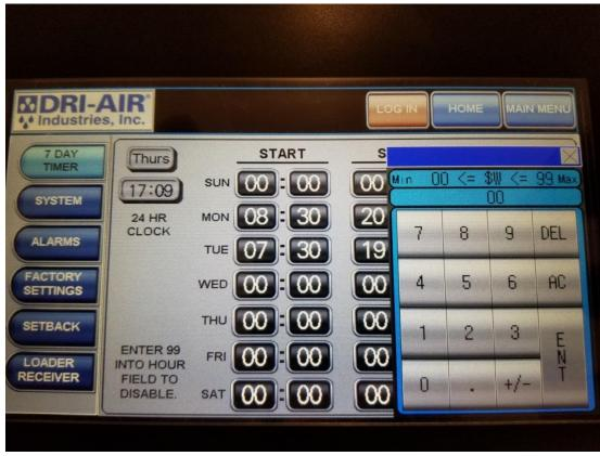
This keypad is used to enter all temperatures, times, and digital information. Press the desired numbers and then ENT to make the change.
