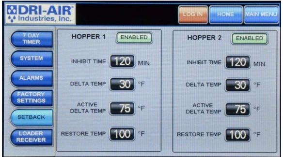
Temperature setback allows the dryer to automatically lower the process temperature after a period of time to keep from over drying the material. Here you can enable or disable the setback as well as setting setback parameters. The factory set parameters will work for most setback applications.
